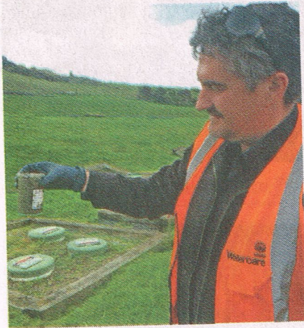
Watercare's wastewater regional manager Jonathan Piggot skims a cup of fat from the Owhanake treatment plant which is struggling to stay within discharge limits. Grease from Oneroa restaurants is thought to be contributing.
